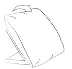
2. To obtain zero position pull the back carefully beyond the top position towards yourself and fold down into zero position (horizontal).
