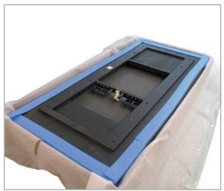
2. Unscrew the 4 feet (a) from the plateau using the Allen key (c) supplied and unscrew also the 2 support feet (b). Lay out the feet and screws (d) removed from the plateau and the screws (d) supplied in front of you.
