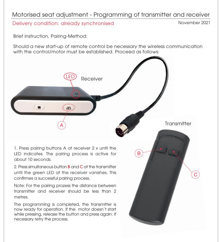
The programming is completed, the transmitter is now ready for operation. If the motor doesn't start while pressing, release the button and press again. If necessary retry the process.
